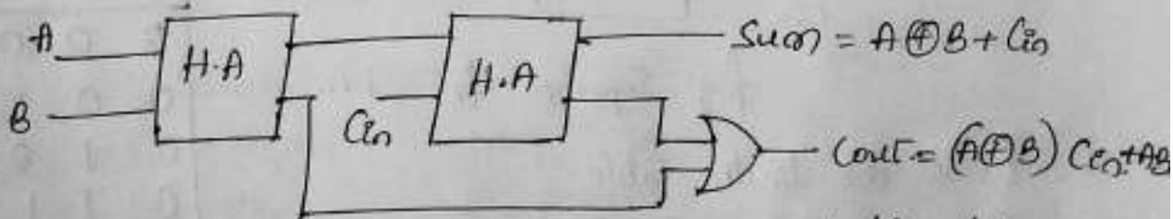
fig: Symbol of full adder using 2 Half adders.
