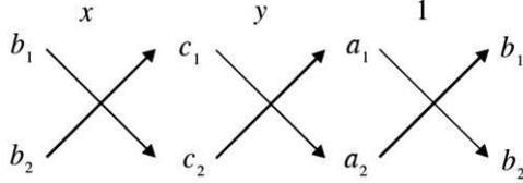
$$\frac{x}{b_1c_2 - b_2c_1} = \frac{y}{c_1a_2 - c_2a_1} = \frac{1}{a_1b_2 - a_2b_1}$$
